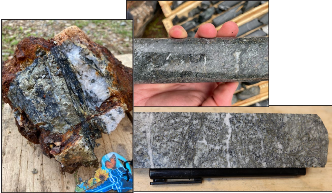
Figure 5: (Left) Outcrop grab sample collected during 2021 prospecting at Elmtree. The sample contains pyrite, arsenopyrite, sphalerite, and galena. (Right) 2021 drill core photos showing pervasive alteration of Fe-bearing mafic minerals. Abundant arsenopyrite throughout which correlates strongly to gold mineralization.
