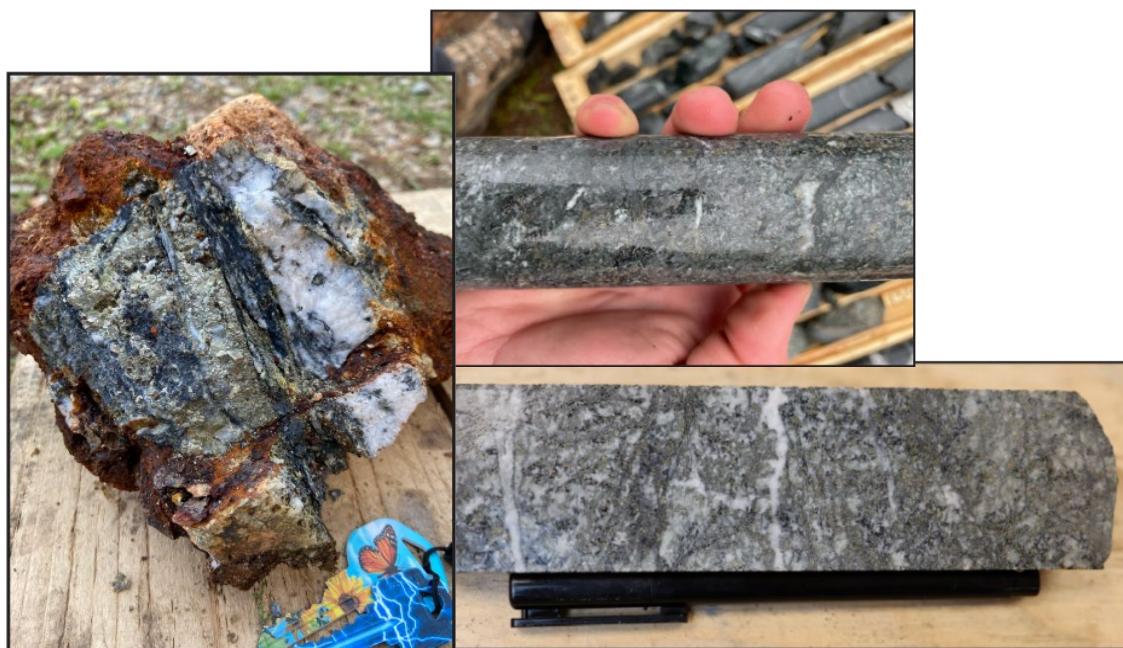
Figure 7: (Left) Outcrop grab sample collected during 2021 prospecting at Elmtree. The sample contains pyrite, arsenopyrite, sphalerite, and galena. (Right) 2021 drill core photos showing pervasive alteration of Fe-bearing mafic minerals and abundant arsenopyrite throughout which correlates strongly to gold mineralization.
