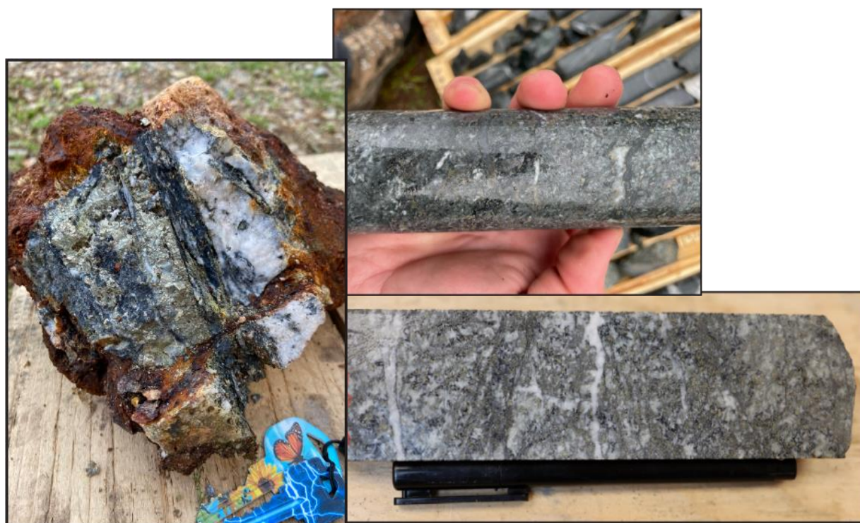
Figure 12: (Left) Outcrop grab sample collected during 2021 prospecting at Elmtree. The sample contains pyrite, arsenopyrite, sphalerite, and galena. (Right) 2021 drill core photos showing pervasive alteration of Fe-bearing mafic minerals and abundant arsenopyrite throughout which correlates strongly to gold mineralization.
