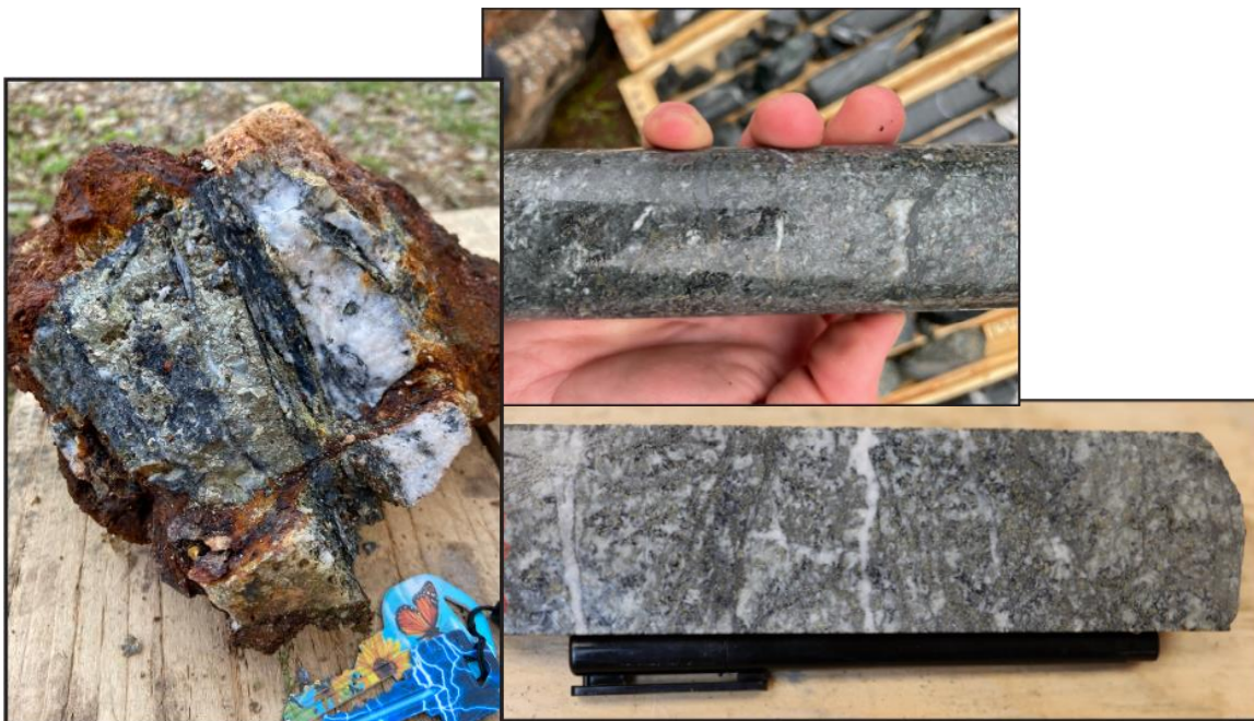
Figure 13: (Left) Outcrop grab sample collected during 2021 prospecting at Elmtree. The sample contains pyrite, arsenopyrite, sphalerite, and galena. (Right) 2021 drill core photos showing pervasive alteration of Fe-bearing mafic minerals and abundant arsenopyrite throughout which correlates strongly to gold mineralization.
