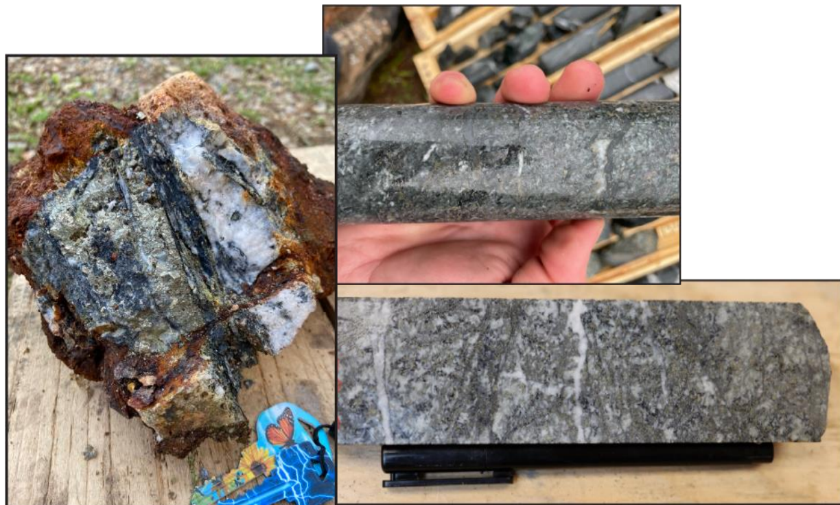
Figure 11: (Left) Outcrop grab sample collected during 2021 prospecting at Elmtree. The sample contains pyrite, arsenopyrite, sphalerite, and galena. (Right) 2021 drill core photos showing pervasive alteration of Fe-bearing mafic minerals and abundant arsenopyrite throughout which correlates strongly to gold mineralization.
