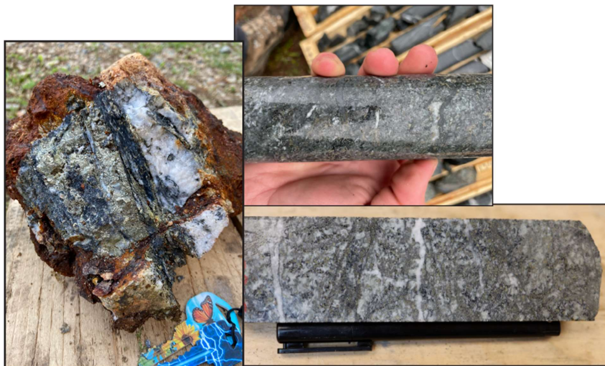
Figure 8: (Left) Outcrop grab sample collected during 2021 prospecting at Elmtree. The sample contains pyrite, arsenopyrite, sphalerite, and galena. (Right) 2021 drill core photos showing pervasive alteration of Fe-bearing mafic minerals and abundant arsenopyrite throughout which correlates strongly to gold mineralization.
