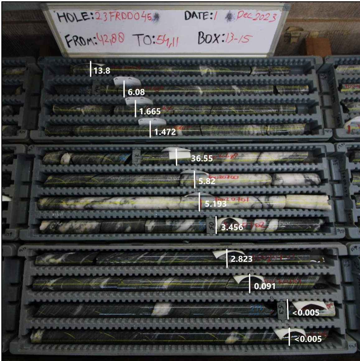
Figure 3. Representative interval of hole 23FR045 gold mineralization in unweathered volcanic rocks below the saprolite/oxide boundary. Gold mineralization is associated with the iron sulphides, pyrrhotite (dominant) & pyrite, as well as strong silicification with substantial quartz veining at the zone's centre. The core shown is from the third gold zone down hole grading 8.54 g/t Au over 9.0 m.
