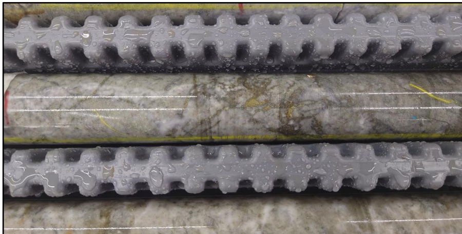
Figure 1: Photo of hole 23DO07 drill core showing alteration and textures common to the highest-grade gold mineralization. Shown is an ~40 cm interval from within a 1 metre interval grading 113.40 g/t Au.
